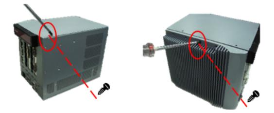
Step 4 After opening the top and side covers, you can locate the CPU socket and heatsink as marked.
